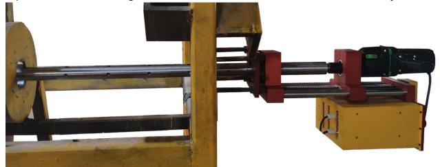
YK60&YKH60 Portable Line Boring Machine is a proven dependable and extremely powerful on-site boringmachine. It offers workshop-quality tolerances on-site and can eliminate costly dismantling and production downtime.
