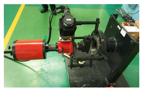
Our TDF400-A portable valve repair machine is a multi-functional equipment. The standard accessory is a turning machine. The optional accessories enable TDF400-A to finish different works.
