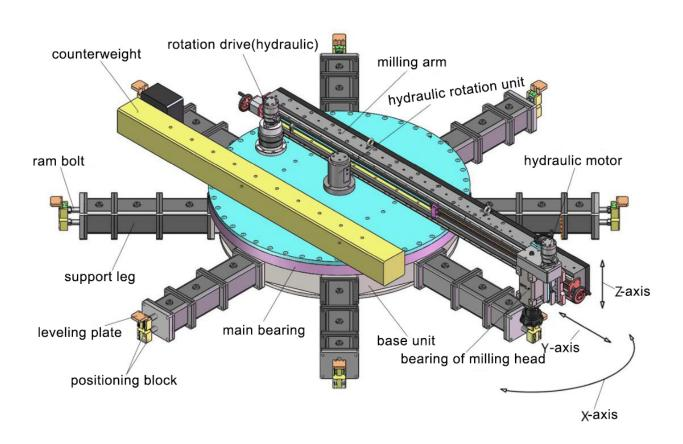
The main rotating power of the equipment is provided by the hydraulic motor, which drives the turntable bearing to rotate through the gear ring gear, thereby driving the milling arm to rotate. A milling power head is installed on the milling arm. The milling power is provided by a hydraulic motor. The milling power head can be manually fed in the radial and vertical directions.
