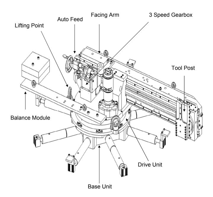
FC2000 Portable Flange Facer is ID mounted design. It can machine flanges up to 86.6"(2200 mm) in diameter. Designed for the rugged challenges of the oil, gas and chemical industry. This flange facing machine allows you to machine all types of flange facing, seal groove machining, weld-prep and counterboring.
