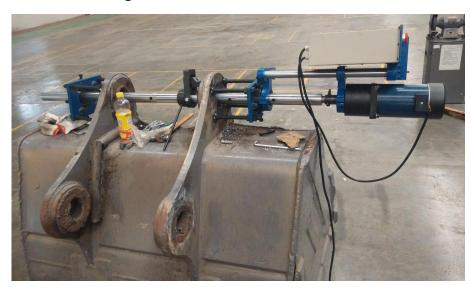
JRT50 Portable Line Boring Machine is a compact, versatile and powerful line boring machine. It can be adapted to variety of the tight space. It is widely used for excavator, loader, bulldozer, crane buckets repair.
